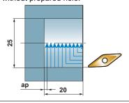
Machining a workpiece with a prepared hole.
