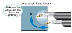
Crossing the center line can chip the insert.
