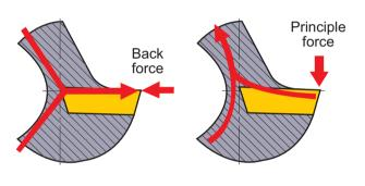
The Dimple bar design effectively balances the principal and back forces, and reduces deflection by up to 17%
