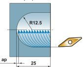
Machining a workpiece with a prepared hole.
