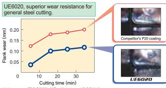
: FSCLP2220L-09E Workpiece : JIS SCM440 Insert : CPMH090304-MV Boring Cutting speed: 180m/min Overhang: 48mm (I/d=3) : 0.15mm/rev Wet cutting Depth of cut : 1.0mm
